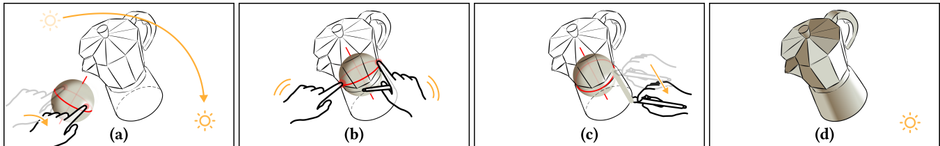
Figure 1: We propose ValueSphere , a novel pen and multi-touch widget designed for quick and easy shading in digital drawings. With ValueSphere , the user can (a) set the light direction, (b) relocate, resize, and rotate the widget to find correct shading values, and (c) apply them to the line sketch in order to achieve (d) plausible volumetric shading.
