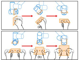
Figure 4: When the handheld virtual plane is translated and rotated, the motion deltas of the handheld plane are transmitted to the end effector in real time. The user can control the end effector as if physically holding and moving it by the planar handle, with (a) one or (b) two hands.
