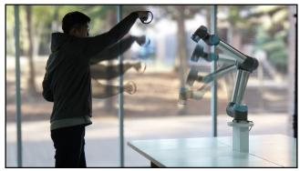
Figure 1: Robot Telekinesis [Lee et al. 2020] allows the user to remotely control the movement of the end effector of a robot arm with hand gestures that closely resemble handling a physical object.
